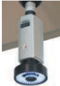
QVP (Sonda para Quick Vision)
